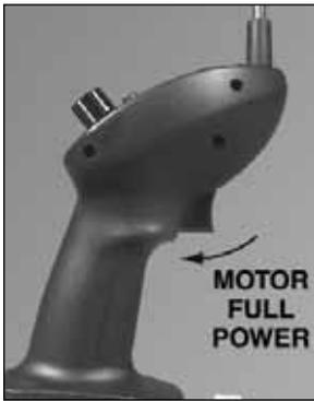
4. Check the operation of the motor and rudder. If either does not operate correctly, **DO NOT FLY**.
