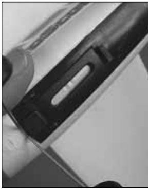
3. Slide the battery into the plane and reattach the battery cover.
