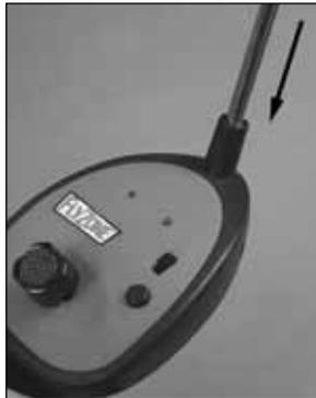
5. Insert the antenna into the top of the transmitter. Turn the antenna clockwise to screw it in place. Do not overtighten antenna.
