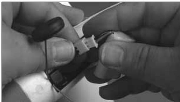
2. Remove the battery cover on the bottom of the plane and connect the battery.
