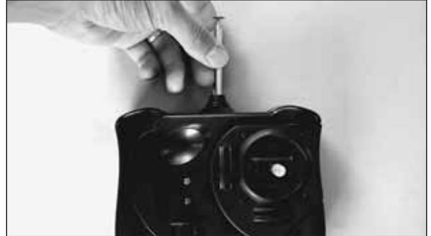
❑ 1. Locate the antenna and screw it into the top of the transmitter.
