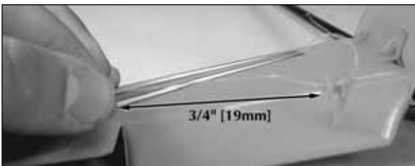
❑ 7. Feed the wire through the hole in the control horn and then through the hole in the adjustment knob. Pull approximately 3/4" [19mm] of excess wire through the knob.
