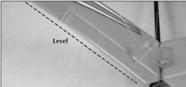
❑ 5. Using the **adjustment knobs** on the **control horns**, adjust each control line until the elevon surfaces are level with V-tail fins.
