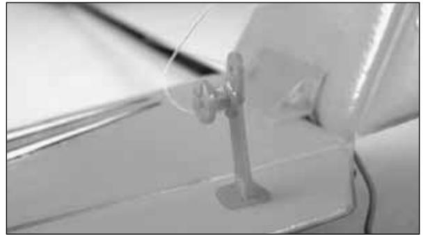
❑ 8. While holding the excess wire taut, rotate the knob so that the wire is reeled in. A few rotations will then keep the wire tight on the knob. Adjust the knob until the elevon is level.
