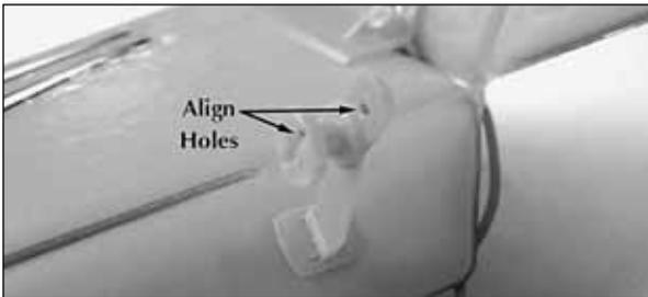
❑ 6. If at any time the control wire needs to be rethreaded onto the adjustment knobs, rotate the knob until the small hole in it aligns with the outer hole in the control horn.
