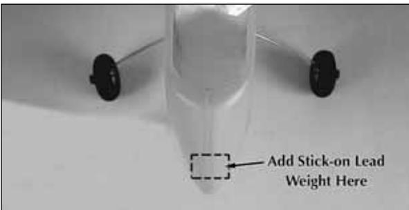
❑ 4. If the model balances with your fingertips **behind** the lines, weight will have to be added to the **nose** to get the model to balance. Nose-weight may be stuck to the upper inside of the fuselage, just in front of the foam
