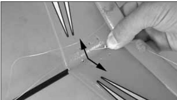
❑ 2. Align the two loops of the **tail wheel wire** with the holes at the back of the fuselage on the bottom. Push the two thumb screws through the two loops in the tail wheel wire and into the **V-tail tray** at the back
