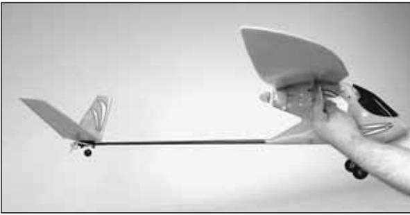
❑ 2. With the battery in place, lift the model with your fingertips between the lines under the wing. Position your fingertips where necessary to get the model to sit level, or “balance.” If your fingertips are between the lines, the Red Hawk is ready to fly.
