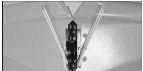
❑ 4. Locate a small rubber band included with the Red Hawk. Hook the rubber band to the left **elevon control hook**. Loop the rubber band around the front of the V-tail tray and connect the rubber band to the right control hook.
