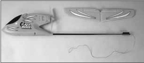
❑ 1. Remove the **fuselage** from the packaging. Be careful when removing the fuselage from the packaging as the **control wire** that is preinstalled in the fuselage is connected to the **V-tail**. Lay the parts out on a table ensuring the control wires are not intertwined or twisted together. Untie the red antenna wire and let it hang freely. **Do not cut off excess antenna wire!**
