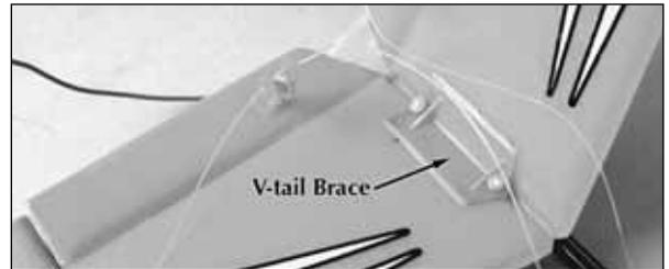
❑ 3. Locate the red plastic **V-tail brace** and align the pegs with the six holes in the V-tail. Secure the brace by turning the thumb screws drawing the brace tight against the tail. If you have difficulty tightening the brace, confirm that the thumb screws are aligned with the two screw holes in the brace. Confirm that the control wires are not pinched underneath the brace. Correct if necessary.
