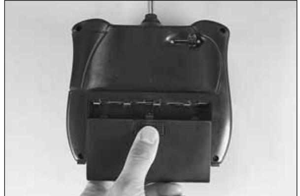
❑ 2. The transmitter that controls your airplane requires power, in the form of eight “AA” batteries. To install the batteries, remove the battery hatch on the back of the transmitter.
