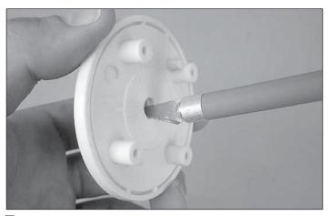
□ 1. Ream the spinner backplate to 5/16" [7.9mm] using a hobby knife, prop reamer, or drill.
