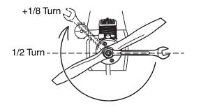
□ 2. Install the backplate, prop, prop washer, and prop nut. Tighten the propeller nut "finger tight," then use a 12mm wrench or a crescent wrench to fully tighten the nut - 1/2 turn, plus 1/8 turn.
