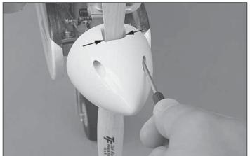
□ 3. Install the spinner cone and tighten the four Phillips screws. Insure the spinner cone does not contact any part of the propeller
