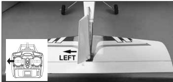
□ 3. Move the left stick to the right and observe the rudder. Moving the left stick to the right should make the rudder (and nose wheel) move to the right. Moving the left stick to the left should make the rudder and nose wheel move in the opposite direction.
