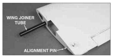
1. Insert the aluminum wing joiner tube in the forward hole in the wing root rib of the left wing half as shown.
