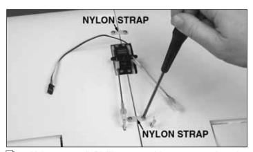
☐ 3. Using a small Phillips screwdriver, secure the wing halves together by installing the two nylon straps with the two 2.3mm x 10mm washer head screws as shown.
