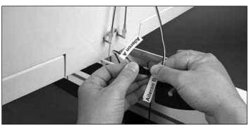
☐ 1. Connect the aileron servo plug labeled "Aileron A" to the plug labeled "Aileron B" coming from the receiver inside the fuse. Do not force them together; they are designed to fit together only one way.
