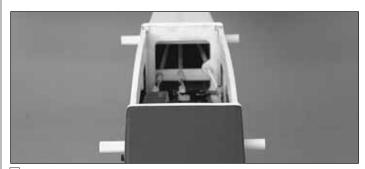
2. Locate the 8mm x 109mm and 8mm x 103mm dowel rods. Insert them through the fuselage as shown with the longer of the two toward the front of the plane. When satisfied with their fit and placement, use CA to secure them in place.
