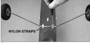
1. Insert the main landing gear wires into the holes in the landing gear blocks in the bottom of the fuse as shown. Secure the gear with the two supplied nylon straps and four 2.5 x 10mm screws.
