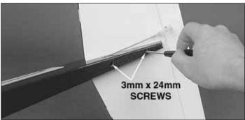
☐ 4. Insert the stabilizer and center it in the stabilizer slot as shown. Use a Phillips screwdriver to install the two 3mm x 24mm screws into the bottom of the fuse as shown to secure the stabilizer.
