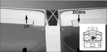
☐ 1. Moving the right control stick on the transmitter to the right, observe the direction the ailerons move. The right aileron should move up and the left aileron should move down. Moving the control stick to the left should make the ailerons move the opposite way.
