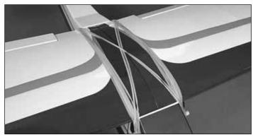
☐ 2. Center the wing atop the "wing saddle" and secure it in place with the included rubber bands. Twelve rubber bands are suggested. It is a good idea to "crisscross" the final two rubber bands. This will help to hold the others in place. Be sure that the electrical wiring is tucked neatly inside the fuse and is not interfering with any of the linkages.
