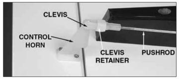
☐ 5. Connect the elevator pushrod into the fourth hole out from the base of the control horn as shown. Slide the silicone clevis retainer in place to help secure the linkage.
