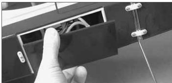
☐ 1. The battery compartment is underneath the fuse, just to the rear of the nose wheel. Gently twist the nylon latches to release the battery door.
