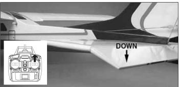
☐ 2. Move the right stick down and observe the direction the elevator moves. Moving the right stick down should make the elevator move up.
