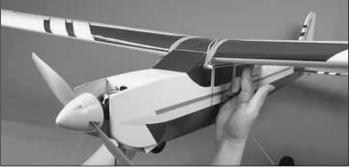
☐ 2. Mount the wing on the fuse with just four rubber bands. Lift the model on both sides of the model with your fingertips
