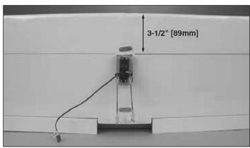
☐ 1. Take the wing off of the fuse and use a felt-tip pen or 1/8" [3mm]-wide tape to accurately mark the balance point located 3-1/2" [89mm] back from the LE as shown in the photo.
