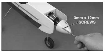
☐ 1. Use a Phillips head screwdriver to remove the two 3mm x 12mm screws from the spinner assembly and gently remove the spinner cone as shown.
