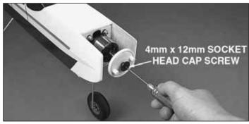
☐ 2. Remove the 4mm x 12mm socket head cap screw and propeller washer from the shaft of the motor.
