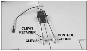
4. Attach the unconnected pushrod to the control horn via the clevis and slide the silicone clevis retainer in place as shown.
