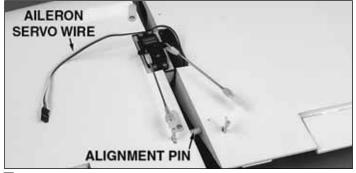
☐ 2. Join the left and right wing halves together making sure that the alignment pin inserts into the opposite wing half. Gently push the wing halves together. Be careful not to crimp or otherwise damage the aileron servo wire.
