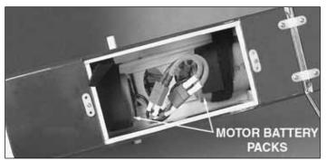
□ 3. Plug the two 7-cell battery packs into the battery connectors. Though it is highly unlikely that the motor will start, stay away from the propeller once the batteries have been plugged in.
