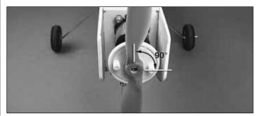
☐ 3. Place the propeller onto the shaft so that the blades are perpendicular to the spinner screw receptacles on the backplate as shown.
