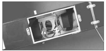
☐ 2. Slide two 7-cell motor battery packs into the battery saddles and secure them with the hook & loop material as shown.
