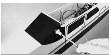
☐ 3. Locate the four plastic dowel rod caps and place them on the ends of the dowel rods that you just installed. Secure each of them with a 2.3mm x 10mm self-tapping washer head screw.
