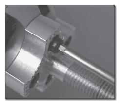
2. Remove the prop adapter by withdrawing the four 3x10mm cap head screws with a 2.5mm hex wrench.
