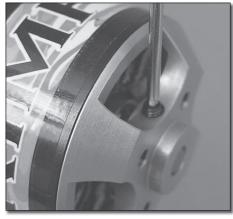
3. Remove the 3mm set screw from the Rimfire with a 1.5mm hex wrench.
