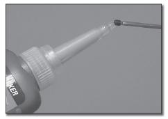
4. For best results, add removable thread locker to the threads on the set screw and reinstall. Repeat this process on the 3x10mm cap head screws and reinstall the prop adapter.
