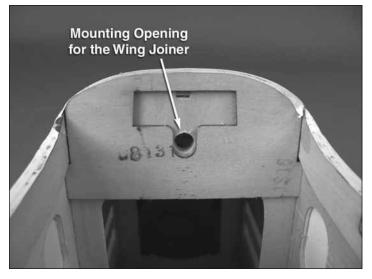
□ 2. In order to make the center core wing joiner more accurately line up at the bolt opening in the rear of the cockpit area, it may be necessary to elongate the mounting opening for the wing joiner.
