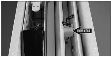
2. Locate the foam block included with the kit contents. If the block is not available, a 1-1/8"x1-1/8"x5/8" [30 x 30 x 15mm] piece of the foam packaging included with the kit would suffice.
