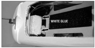
3. Press the block in place against the protruding screw tips. Use white glue to hold the block in place.
