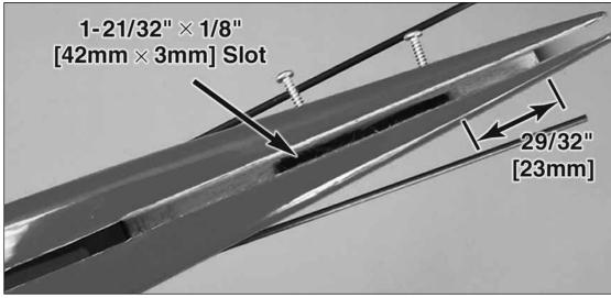
**Before** installing the tail surfaces, it may be necessary to cut a  $1-21/32" \times 1/8"$  [42mm  $\times$  3mm] slot at a distance 29/32" [23mm] from the rear of the fuselage, to accept the longer tab on the vertical stabilizer.
