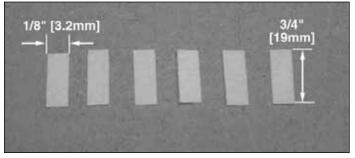
□ 21. Cut six hinges out of the CA Hinge material 1/8" [3mm] wide by 3/4" [19mm] long.
