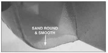
□ 35. Sand the inner edge of the inlet smooth. This is important to improve the fan's performance.
