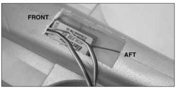
□ 17. Connect the servo wires to the receiver and slide the receiver in place as shown above. Connect the servos to channel 1 and 2 and set up an elevon mix in your transmitter. Make a small hole in the aft area of the fuselage and route the antenna wire out of the fuselage. **Warning**: Let any excess antenna wire hang at the back of the fuselage. Do not coil it up inside the fuselage and do not cut it to length.
