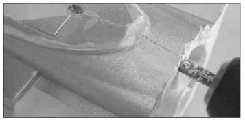
$\Box$  9. Use a 1/4" [6mm] drill bit to drill a hole as shown above. This hole is for the SC battery wire.
