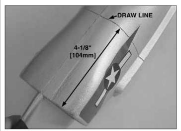
□ 3. Draw a line at the bottom of the fuselage 4-1/8" [104mm] away from the duct entry. Continue this line around the fuselage as shown above.
