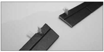
□ 25. Cut a slot in the elevators at the mark. Glue the control horns in place with foam-safe CA or epoxy. The control horns should be facing the upper side of the elevators.
