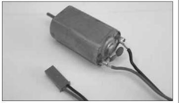
□ 11.Locate the speed control. Cut the connector on the motor end of the speed control and solder it to the motor. The red wire goes to the motor tab with the red dot. Make sure the wires are 1-3/4" [44mm] long.
