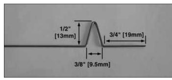
□ 28. Bend one end of both .035" [0.9mm] pushrod wires as shown above. Cut the other end of one of both pushrods wires 10" [254mm] long to make both elevon pushrods.
