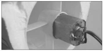
□ 12. Insert the motor into the housing. Apply some epoxy or CA to glue the motor in place. Also, re-install the fan blade on the motor axle by applying some CA onto it.
