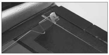
□ 30. Cut a small portion of the leftover CA Hinge material and make a small hole in it. Place it against the control horn as shown above. Use a drop of medium CA on the CA Hinge material to glue it to the pushrod. Make sure you do not glue the CA hinge material to the control horn.
