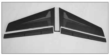
□ 20. Locate the stab. Draw a line 1/2" [13mm] forward of where the elevator hinge line is and cut the elevators out with a sharp #11 blade.
