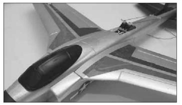
□ 34. Remove the protecting film on the wing's and fuselage's double-sided tape. Apply some foam safe CA to the gluing area and install the wing in place. Let the glue cure.
