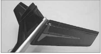
□ 27. Remove the protecting film on the double-sided tape on the stab and on the fuselage and press the stab in place.
