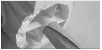
□ 6. Sand the inner side of the housing until the new motor fits in. The fit should be snug.
