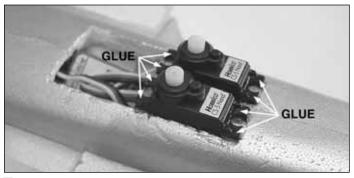
□ 19. Install the servos as shown above. Apply a drop of CA on each mounting arm to glue them in place.
