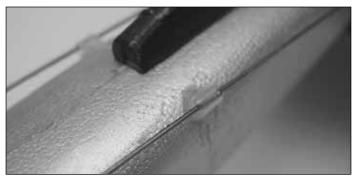
□ 32. Lightly sand the plastic tube on the pushrod and then glue it with foam-safe CA to the fuselage of the airplane to prevent the pushrod from bending under load.
