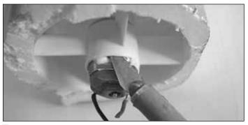
□ 5. Remove the motor from its housing using a hobby knife and then discard it.
