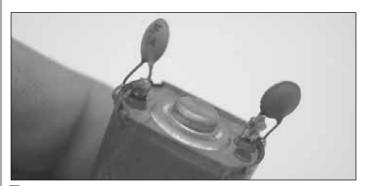
□ 10. Locate the motor and two capacitors. Solder one leg of each one of the capacitors to a motor power tab and the other to the motor case.
