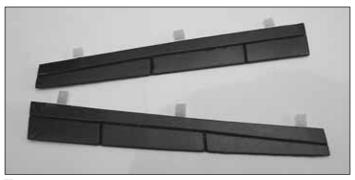
□ 23. Apply some foam safe CA to half of each hinge. Slide three CA hinges in place in the elevator. Let the CA cure.
