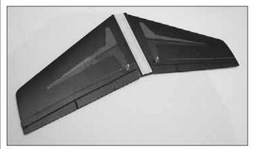
$\Box$  26. Apply foam safe CA or epoxy to the elevators' hinges and slide them into the stab. Let the glue cure. There must be at least a 1/16" [1.6mm] gap between the surfaces.
