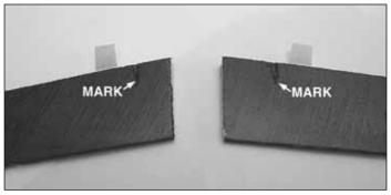
□ 24. Mark the location of the two elevator control horns as shown above.
