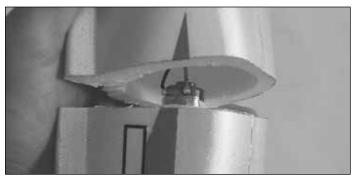
□ 4. Use a hobby knife with a sharp #11 blade to cut the fuselage in two at the lines. Also, cut the motor wires with a wire cutter.
