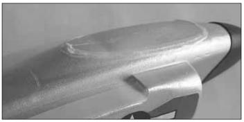
2. Carefully separate the canopy from the fuselage using a hobby knife.
