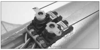
□ 31. Install the pushrods onto the servo arm. Make sure the servo arms are 90 degrees to the servo.
