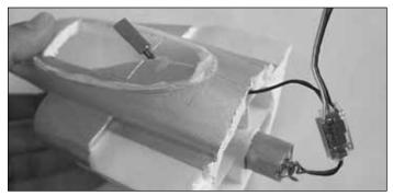
□ 13. Slide the SC battery wire into the hole drilled in step 9. Apply some double-sided tape to the flat side of the SC.
