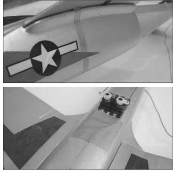
□ 36. Apply some colored tape on the fuselage's glue joints. Use tape to hold the canopy in place. The finished weigh of your airplane should be between 7.7 and 8.3 oz [220 and 235g].
