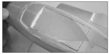
□ 8. Using the lines as guides, cut the top of the fuselage open, being careful not to cut into the duct. This will be the battery compartment. Check the image above for reference.
