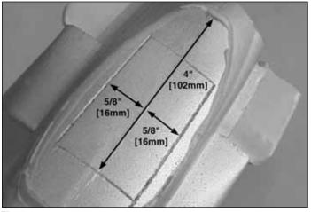
$\Box$  7. Draw a line perpendicular to the fuselage axis approximately 4" [102mm] from the aft edge of the canopy.
