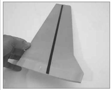
$\square$  33. Glue a strip of carbon fiber to the bottom of both wings.
