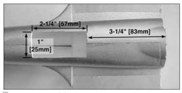
□ 14. Locate the aft fuselage and cut a rectangular opening 1" x 2-1/4" [25mm x 57mm] 3-1/4" [83mm] away from the cut end of the fuselage. Remove the FF battery.
