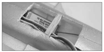
□ 18. Cut a 1/8" [3mm] piece of balsa 1/8" [3mm] wide by 1" [25mm] long. Glue it 7/8" [22mm] in front of the aft edge
