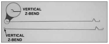
□ 29. Slide a small tube 1/4" [6mm] long (such as an ink pen tube) on each pushrod. Make a "Z-bend" at the long end of both pushrods as shown above. Also, bend both short ends of the pushrod. The Z-bends are 90° to the work surface.
