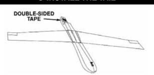
Remove the backing from the double-sided tape on each side of the fuselage for the tail as shown.
