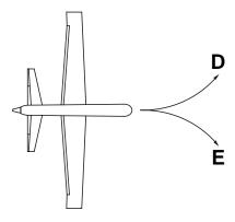
**D** = To turn left, bend the left ruddervator down slightly and the right ruddervator up slightly.
