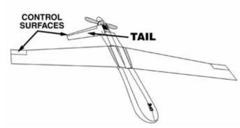
Attach both stabilizer halves to the fuselage. The control surfaces need to face the propeller.
