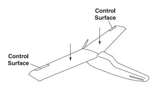
• Attach the main wing halves to the fuselage by lining them up along the centerline of the fuselage. Control surface should face the propeller.
