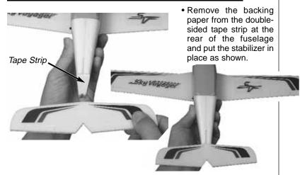
Locate the two (2) strips of tape in the accessory bag. Press-fit the vertical fin in place and secure it to the fuselage by putting a strip of tape on either side of the rudder as shown.
