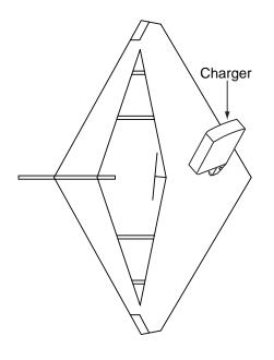
4. Push and hold the charge button on the charger. On the first charge, only charge the Regent for 15 seconds. For longer flights, you may increase the charge time up to 60 seconds.
