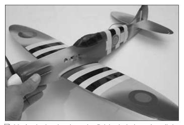
□ 38. Apply the decals to the finished airplane. Install the propeller. The ready-to-fly weight should be between 6.3oz and 6.7oz [180 - 190g].
