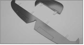
□ 13. Apply some foam-safe CA to half of each hinge. Slide two CA hinges in place in the rudder and four in the elevators. Let the glue cure.
