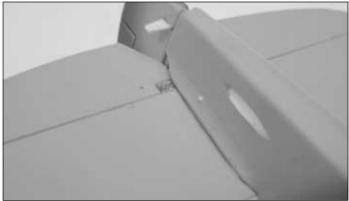
□ 17. Use a small drill or a sharpened brass tube to make a hole approximately 3/32"[2.3mm] into the fuselage sides for the elevator and rudder pushrods.
