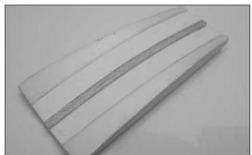
□ 29. Locate the belly pan. Lightly sand the plastic where the wing is to be glued on. Cut a 1/8" [3.2mm] strip of 1/16"[1.6mm] balsa and glue it on to the centerline as shown above. This is done to modify the wing dihedral. Sand the balsa wood and fit the two wings onto the belly pan until the dihedral is 3-9/16" [90 mm] measured with one wing flat on the work surface with the belly pan installed.
