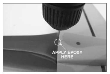
□ 36. With the wing in place, drill a 1/16"[1.6mm] hole between the trailing edge of the wing and the fuselage at the center section of the wing. Remove the wing. Mix a small amount of epoxy and apply it to the hole area. Also, apply some epoxy to the trailing edge of the wing.
