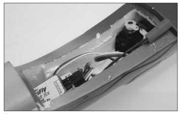
□ 27. Install the frequency crystal to the receiver. Connect the speed control and the servos to the receiver. Route the receiver antenna to the back of the fuselage and out of the fuselage. Install the receiver into the forward area of the fuselage.
