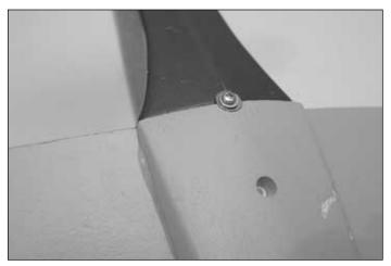
□ 37. Install the wing in place with one #2 x 1/2" [12mm] screw and a #4 washer.
