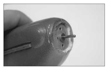
□ 26. Slide the speed control and the motor into the fuselage through the hole in the front where the other motor was. The motor should fit snug. You may have to trim the opening slightly for the motor to fit well. Apply a dab of epoxy to glue the motor in place. Make sure you glue it in with the original downthrust and right thrust noted in step 7 on page 2.
