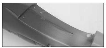
□ 2. Carefully remove the double-sided tape from the fuselage's wing saddle.
