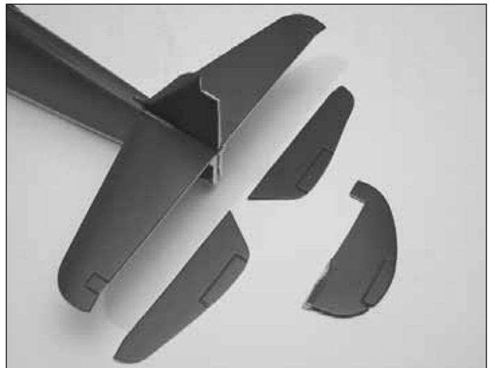
❑ 8. Cut the rudder off of the fin at the hinge line using a hobby knife with a sharp #11 knife. Lightly sand the cut edges with 400-grit sandpaper. Cut the elevators off of the stabilizer at the hinge line and sand the edges.
