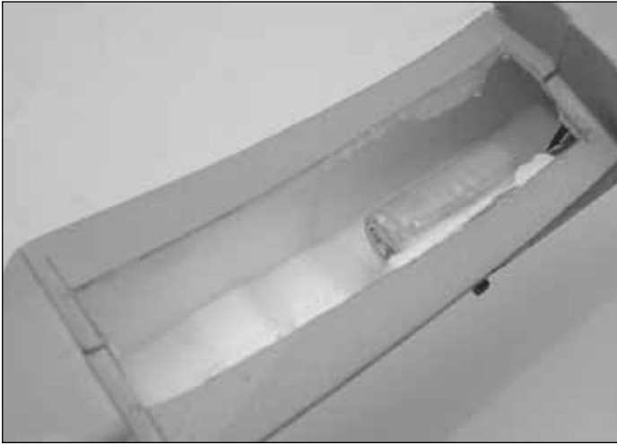
❑ 4. Use a hobby knife with a sharp #11 blade to cut the fuselage open at the lines.
