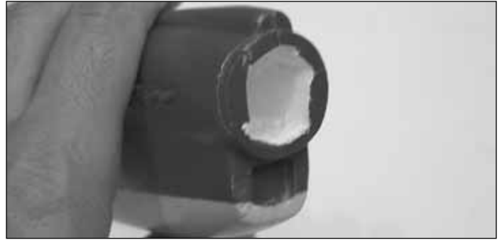
❑ 7. Measure the current motor right thrust and down thrust. Then, discard the motor. Use a hobby knife to cut the motor out of the fuselage.
