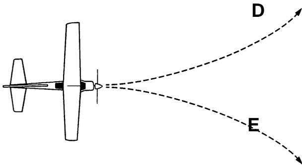
**D** = To turn left, bend the rudder slightly to the left.
