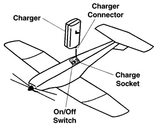
4. On the first charge, only charge the airplane for 15 seconds. For longer flights, you may increase the charge time up to 60 seconds.
