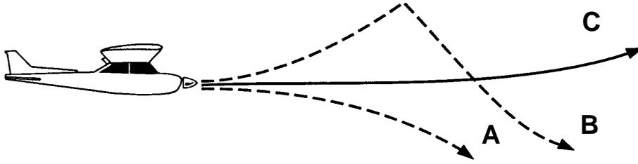
**A** = Dive. Bend elevators upward slightly.
