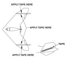
2. Remove the backing from the clear tape and apply it to the joint between the fin and wing.
