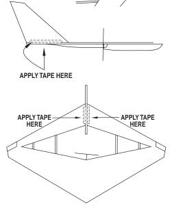
2. Remove the backing from the clear tape and apply it to the joint between the fin and the wing and to the underside of the wing where the fin slides into the wing.
