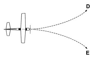
**D** = To turn left, bend the rudder slightly to the left.
