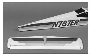
□ 14. Using a hobby knife, cut inside the lines made with a felt-tip pen and remove the covering from the center of the horizontal stabilizer. **Do not** cut into the balsa sheeting on the horizontal stabilizer.
