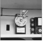
The throttle servo horn should move 40Þto the rear.
