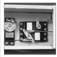
The rudder servo horn should rotate counter clockwise.
