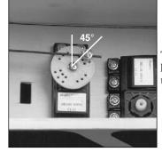
The throttle servo horn should be 45P to the rear.
