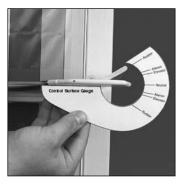
The rudder should move to the right as shown on the surface control gauge.
