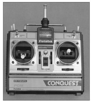
□ 8. With the radio system on, move the throttle stick down (idle position) and the throttle trim up. All other trim and stick controls should be moved to their neutral positions.
