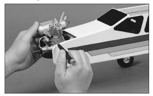
□ 2. Locate the *muffler* and mount it to the engine by using two 3 x 30mm machine screws. The exhaust outlet should be pointing down and away from the fuselage.
