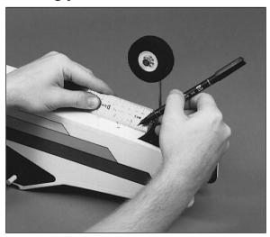
□ 36 Using a felt-tip pen, place a mark 5/16" (8mm) from the engine compartment and 1" (25.5mm) from the side of the fuselage on the bottom of the fuselage.
