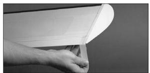
$\Box$  22. Use masking tape to hold the ailerons in the neutral position while connecting the servo linkages.
