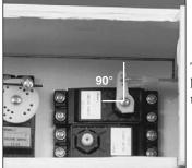
The elevator servo horn should be 90P to the servo.
