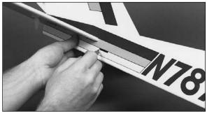
□ 28. The precut elevator pushrod exit hole is located on the same side of the fuselage as the elevator control horn, beneath the covering 1/2" (12.5mm) in front of the horizontal stabilizer. Locate the exit hole by gently running your finger down the side of the fuselage over the covering. Using a hobby knife, remove the covering from the elevator pushrod exit hole. **Do not** remove the covering from the exit hole on the opposite side of the fuselage.
