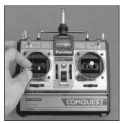
To turn the plane left, move the rudder stick to the left.
