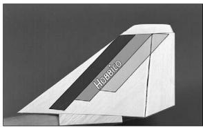
□ 18. <u>Cutting below the line and through the</u> <u>covering only</u>, remove the covering from the base of the vertical fin. **Do not** cut into the balsa fin root.
