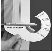
The rudder should move to the left as shown on the control surface gauge.
