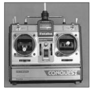
To stop the engine, move the throttle stick back and the throttle trim back.
