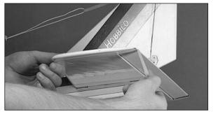
□ 15. Use masking tape to hold the elevator in the neutral position while installing the pushrod and connecting the servo linkage.
