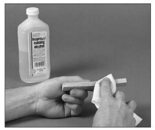
□ 5. Excess epoxy will be squeezed out of the seams between the joiners and must be removed **before** the epoxy is allowed to cure. Use a paper towel and rubbing alcohol to remove the excess epoxy. Be careful not to disturb the alignment of the joiner pieces.
