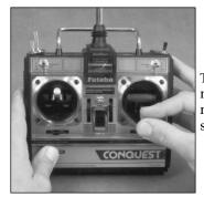
To gain altitude, or make the plane rise, move the elevator stick back.
