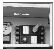
The servo horn should move towards the rear.
