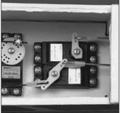
The rudder servo horn should rotate clockwise.
