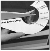
The left aileron will move up as shown on the surface control gauge. The right aileron will move down.
