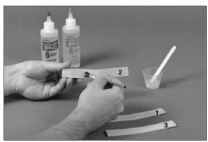
□ 3. Mix approximately 1/4oz. (7.5ml) of 6-minute epoxy. Using a mixing stick or epoxy brush, apply an even coat of epoxy on both sides of the #2 wing joiner. With the #3 wing joiner laying flat on the work surface, stack #2 on top of #3 and #1 on the top of #2. Note: The epoxy should be in between the layers of the plywood wing joiners and not on the outside surfaces.
