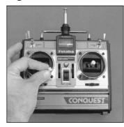
To turn the plane right, move the rudder stick to the right.
