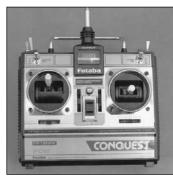
For full throttle, move the throttle stick and trim forward. If the servo horn moves in the wrong direction, switch the reversing switch for the throttle on the *transmitter* or use a reversed rotation servo.
