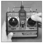
To lose altitude, or make the plane go down, move the elevator stick forward.
