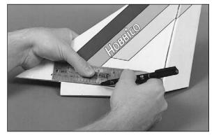
□ 17. Locate the vertical stabilizer. Draw a line on both sides even with the bottom of the fin.
