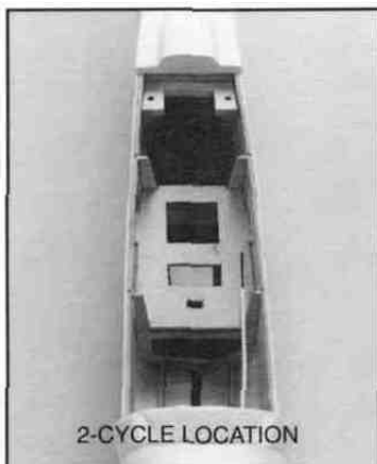
8 If you installed a 2-Cycle engine use the forward most mounting location. If a 4-cycle engine is used mount the servo tray in the rear position. After the proper location is determined epoxy the servo tray in place.
