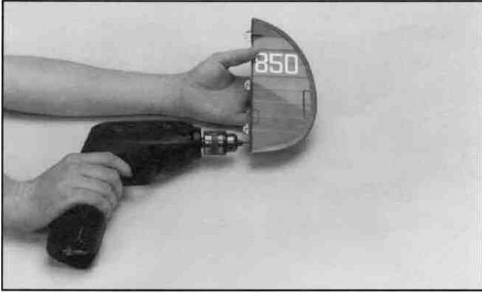
13. Next drill a 1/16" hole about 1" deep at 7/8" from the bottom of the rudder. The hole should be straight in from the front edge.
