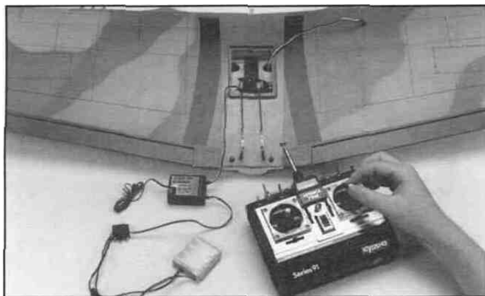
7 Connect the aileron servo to the receiver and check the movement of the ailerons. Make sure that both ailerons are neutral when the servo is neutral. Adjust the clevises as needed.
