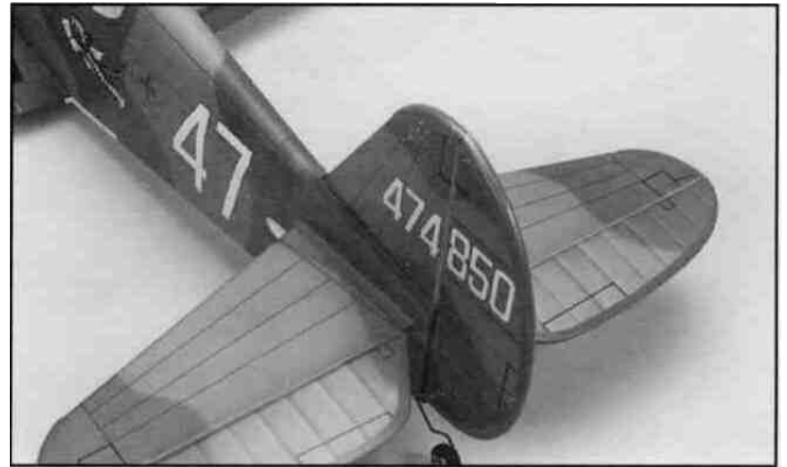
16. Carefully position the tail control rod into the hole and the groove. Wipe off any excess epoxy and then insert the hinges into the slots. Wipe off any excess epoxy from the hinges and check for free operation. Let cure.
