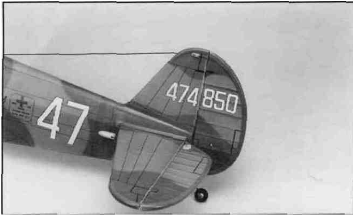
5. Use the plastic antenna retainer and secure the wire to the tail.
