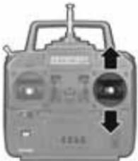
Moving the right stick up or down changes the pitch of the aircraft. Pulling the stick back, for example, causes the **elevator** control to rise — forcing the nose to point up and thereby increasing altitude.
