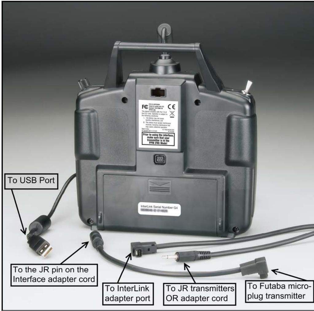
Locate the cable input port on the rear of the InterLink Elite Controller. Plug one end of the included connector cable into this port. Next, plug the other end of the adapter cable into the buddy box port (a.k.a. trainer jack) of your transmitter. The procedure for doing so depends on your transmitter:
