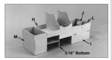
Fit the 3/16" bottom to the assembly, then glue it only to **H**, **I**, **L** and **M** (back, front and sides).
