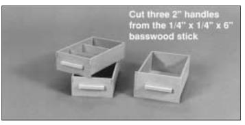
□ Sand the fronts of the drawers so they are flat and smooth. Cut the 1/4" x 1/4" x 6" basswood stick into three 2" pieces, then glue one "handle" to the front of each drawer.
