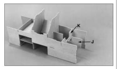
☐ Fit J and K together, then install but **do not glue** them to the assembly. Glue the left side L (see the following photo), to J, H and I and then the right side M to H and I.
