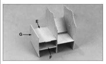
□ Fit E and F to G, then join to C. Note: The notch in F goes toward the rear. Glue the assembly together.
