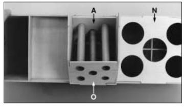
☐ Test fit, then glue **N** in position. Accurately cut the paper tubes in half. Fit but do not glue the paper tubes through the holes in **O** so the "square end" (the end cut by the factory), will be at the bottom and contact **A**. Adjust the paper tubes so they are perpendicular to **O** and **A** and are parallel to each other. Glue the paper tubes to **O** and **A** and then Glue **O** into position.
