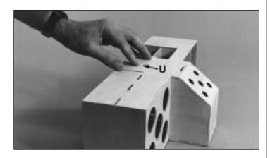
Glue the drawer front **U** to the front edges of **R** and **T** while the drawer is in the BenchTopper. Hint: Place a piece of 1/16" scrap balsa or similar behind the drawer so you do not inadvertently glue the drawer front to the BenchTopper.
