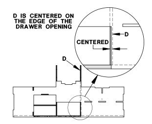
$\Box$  Adjust **D** so it is centered on the edge of the opening for the large drawer. Glue **D** to **I** in this position. Glue all other joints not previously glued.
