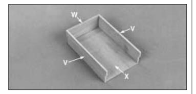
▲ Make two drawers from the sides V, back W, and bottom X. Glue all of the pieces together. Glue the front Y to one drawer and the front Z to the other drawer. The drawer with the front Y is the top drawer and the drawer with the front Z is the bottom drawer. Test fit the drawers and make any adjustments if necessary. **Caution:** The tabs on V are offset and will fit X properly only one way
