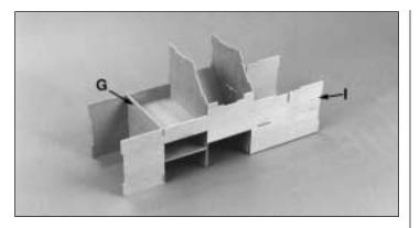
Fit the front I to the assembly. Glue I only to G at this time.
