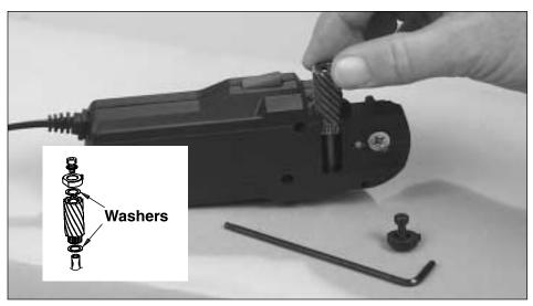
2. Gently and carefully lift the cutting drum straight off the cutter shaft and out of the planer body. The bronze gear on the cutter drum is part of the assembly and not removable. There are washers between the cutter and case. **Do not lose these washers!** They must be reinstalled with the new cutter drum.
