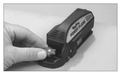
Turning the depth adjustment knob clockwise will increase the cutting depth. The maximum depth of the Power Plane is .030" [.76mm].
