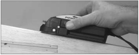
The Power Plane removes material by means of an electrically powered spiral-blade rotary cutter. The cutter
