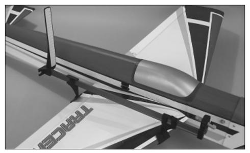
**3.** Without bumping the laser assembly, attach the meter to the wing close to the fuse-lage. If the meter is attached to an aileron, make sure the aileron stays at neutral.
