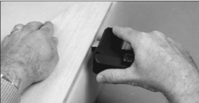
**This photo shows the proper grip to use when operating the Slot Machine.**
