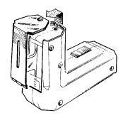
**4**. Remove the blade access hatch by sliding it forward and down.
