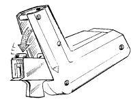
**6**. Pivot the blades and blade holders down and out of the housing.
