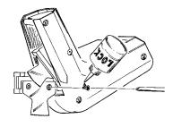
10. Insert a new blade into the blade holder with the 45-degree angled corner matching that of the pocket in the blade holder.
