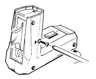
**5**. Remove the rear Phillips head screw (above and slightly to the rear of the blades).
