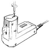
**3**. Remove the front Phillips head screw on the end of the housing.
