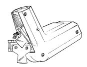
**8**. Pivot one of the blade holders up and out of the way, exposing the blade attachment screws.
