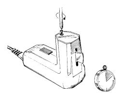
**16**. Reinstall the front Phillips head screw. This screw must engage the dog on the top of the blade holder guide. Tighten securely, but do not over tighten. After installing new blades, we recommend that you allow 2 hours or more for the thread locking compound to set before using the unit to cut slots.
