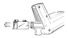
**7.** Slide the blade holder guide off of the blade holders.
