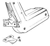
**9.** Remove the blade attachment screws and remove the blade. Notice that one corner of the blade has a 45-degree angle, and note the direction of that angled corner.
