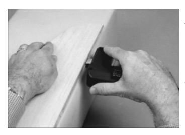
This photo shows the proper grip to use when operating the Slot Machine.
