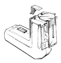
**15**. Insert the blades through the slot in the blade access hatch and snap the hatch into place.
