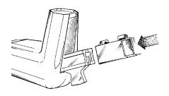
**13**. Slide the blade holder guide back over the blade holders.
