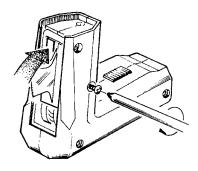
**14**. Pivot the blade assembly up into the housing. Reinstall the rear Phillips head screw through the housing and through the dog on the top of the rear blade holder guide. Tighten snugly, but do not over tighten.
