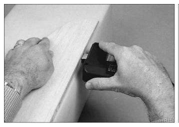
This photo shows the proper grip to use when operating the Slot Machine.
