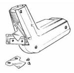
**9.** Remove the blade attachment screws and remove the blade. Notice that one corner of the blade has a 45° angle, and note the direction of that angled corner.
