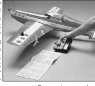
system to obtain the proper output. Remember, moving the connector out on the *servo arm* creates more throw, but moving the connector out on the *control horn* of the control surface creates less throw.
