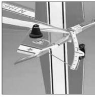
fuselage 90 degrees and attach the unit to the vertical fin in the same manner you would on a stabilizer or wing.
