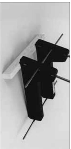
**Note:** In some cases, especially with high-wing tail draggers, the landing gear may interfere with the upright rods. If that is the case, turn the C.G. Machine 180° and switch the socket cap and ruler assemblies. If this does not work, raise the front or back of the bases to change the angle of the upright rods in relation to your airplane, but not enough to make the bases unstable.
