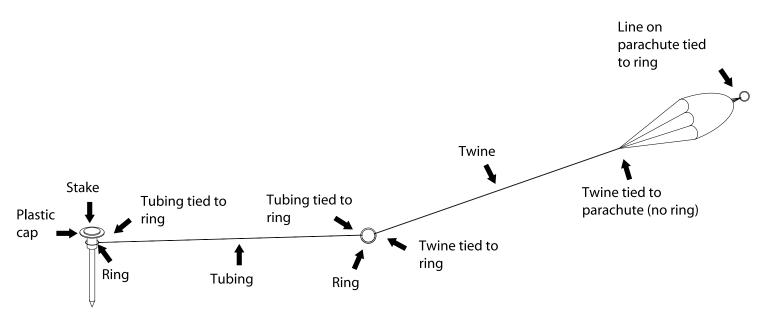
Note: You may need to file the flanges on the tip of metal stake if plastic stake cap does not fit easily.
