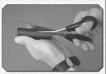
○ 7. Cut the foam cushion tubing into six 3-1/2" [90mm] pieces. Slit each one all the way down.
