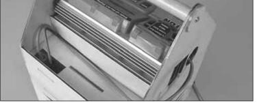
□ 3. Install the handle and the screws. Cut the charger's battery wire to length and solder banana plugs on it. Plug the charger in. Be certain to match wire and plug colors to respect polarity. To turn the Triton charger off, unplug one of the leads.
