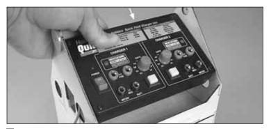
□ 2. Spread the sides of the box slightly, to allow the charger to slide down, then slide the charger into position.
