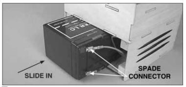
□ 1. Slide the sealed battery into the bottom of the Compact E-Box, connect the spade connectors to the battery and replace the hatch screws. Note the polarity of the battery (red spade connector goes with red wire and positive battery terminal).
