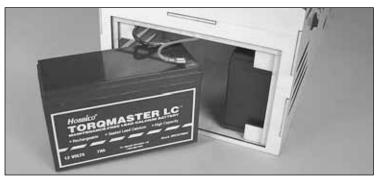
1. Slide one or two sealed batteries into the battery compartment. Connect the spade connectors to the batteries. Note the polarity of the batteries (the red spade connectors go with the red wires and positive battery terminals)
