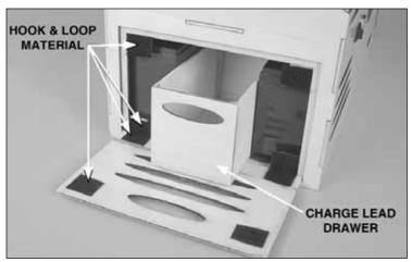
☐ 2. Replace the charge lead drawer. Cut four 3/4" x 3/4" [19mm x 19mm] pieces of hook and loop material. Remove the protecting
