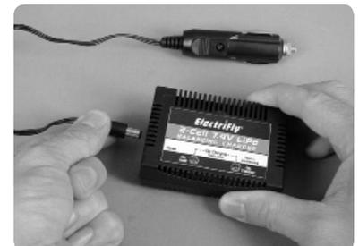
3. When the battery is fully charged, the GREEN LED will turn OFF. Remove the battery from the charger at this time.
