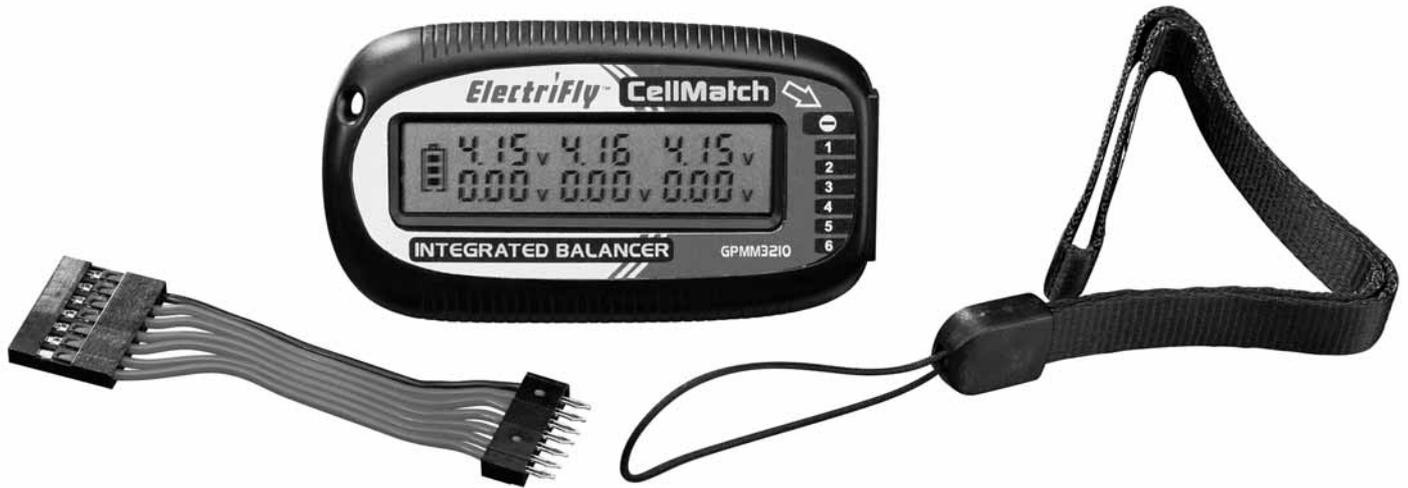
The ElectriFly® **CellMatch** is a precision measurement tool for Lithium-Polymer and Lithium-Ion batteries. This device measures and displays individual cell voltages and remaining battery power. **CellMatch** also identifies voltage differences between cells and discharge-balances all cells. No external power source is needed. It accepts ElectriFly style connectors with 3-7 pins, and includes a 6S in-line adapter for FlightPower® and Thunder Power batteries and wrist strap.
