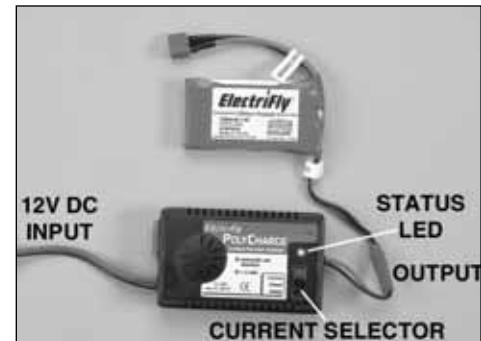
**Input Power and Connector:** Connect the charger to the desired power source using the alligator clips on the input lead as described above. There is no on/off power switch on this charger. Therefore, once connected to input power the charger is active and in "idle mode," ready to be connected to a battery. The bright blue LED will flash once every 3 seconds and the buzzer will beep briefly to indicate that power is applied.
