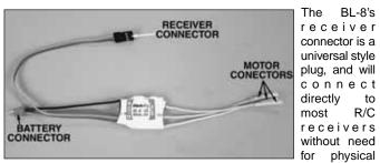
modification or re-wiring. The orange "signal" wire on the ESC's receiver plug should be in the same position in the receiver slot as the white wire on Futaba<sup>®</sup>, the blue wire on the newer Airtronics "Z" connector, the yellow wire on the Hitec "S" connector, or the orange wire on the JR connector. **WARNING:** This connector is NOT directly compatible with the old Airtronics connector style. Use an Airtronics Servo Adapter to connect this ESC to the older style Airtronics radios.
