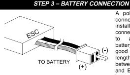
A polarized micro connector is preinstalled for connecting the ESC an external battery pack. It's a good idea for the length of wire between the battery and ESC to be no lonaer than 6
