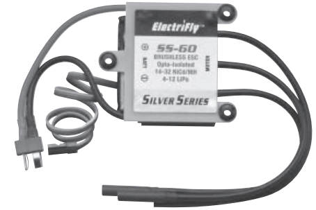
Silver Series 60 (SS-60) ESC (GPMM1850) for 60A maximum constant current draw.
