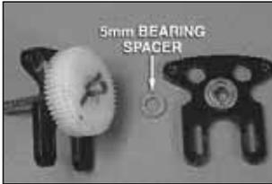
To remove the spur gear, loosen and remove the two 2.5x17mm flat head machine screws and 5.5mm aluminum spacers. Remove the backplate being careful to not lose the 5mm bearing spacer.
