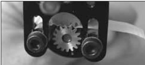
Loosely mount the motor to the back of the back plate with two 3x20mm SHC screws and two 3mm flat washers. Place
