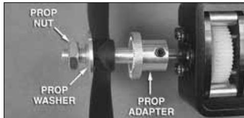
Slide the prop adapter over the output shaft of the gear drive or motor. Align one of the set screws with the flat on the output shaft of the gear drive. Apply a drop of Great Planes **Threadlocker (GPMR6060)** to the set screw and install it in the prop adapter, tightening it against the flat of the gear drive output shaft. Remove the second set screw that does not tighten onto the flat. When installing the prop
