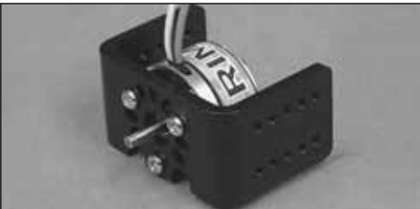
Out-runner motors can be mounted inside the front plate in some situations using three 3x8mm SHC screws, but most of the time they will be mounted on the front of the front plate.
