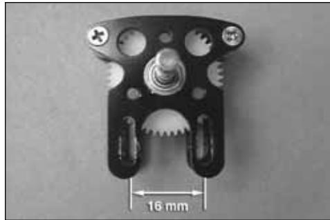
The ElectriFly Ammo motors have high kVs meaning that they like to run at very high rpm. A gear drive is used in order to reduce the rpm allowing a larger, more efficient propeller to be used. Great Planes ElectriFly offers a **24mm Small Gear Drive (GPMG0505)** with several pinions that allow for the following gear ratios:
