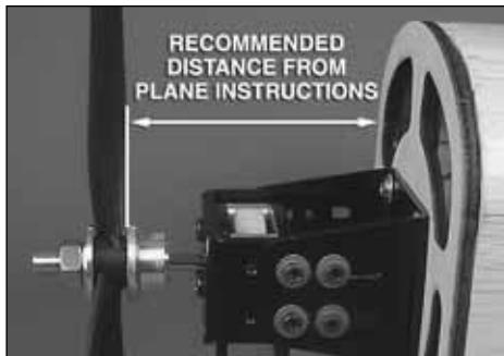
Determine the distance the prop adapter needs to be from the firewall by using the recommended distance in the instructions or by installing the cowl and measuring the distance from the firewall to the front of the cowl. Add approximately 3/32" to 1/8" to the distance. Attach the Front Plate of the motor mount to the Back Plate using the eight 4-40x1/4" SHC screws and eight #4 flat washers, spaced out as far as possible. A drop of threadlocker on the screws will prevent them from coming loose.
