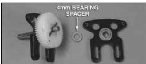
To remove the spur gear, loosen and remove the two 2.5x17mm flat head machine screws and 5.5mm aluminum spacers. Remove the backplate, being careful to not lose the 4mm bearing spacer.
