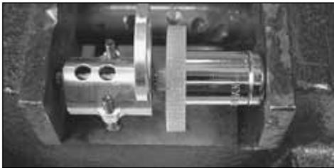
To accomplish this, use a tube or socket placed over the output shaft and against the new spur gear. Place this assembly in a vise and press the gear over the spline.
