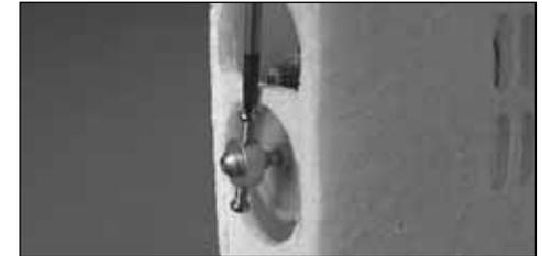
Install the cowl if the plane comes with one. Note that on the prop saver hub the center protrusions have different diameters on each side of the hub. Determine which diameter fits the prop you are using. Then, install the prop saver hub on the output shaft of the gear drive with the correct diameter facing outward. Tighten the two 2.5x7mm machine screws in the prop saver hub against the output shaft.
