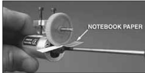
Loosely mount the motor to the back of the gear drive motor plate with two 2.5x4mm machine screws and two 2.5mm flat washers. Place a piece of notebook paper between the pinion gear and the spur gear. Squeeze the two gears together while tightening the two 2.5x4mm machine screws. Remove the piece of paper and the gear mesh is set.
