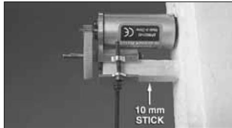
The Great Planes Stick Mount Gear Drive is designed to be mounted on a 10mm stick. Loosen the two 2.5x20mm SHC screws and raise the Top Plate. Slide the Gear Drive over the 10mm stick and tighten the two 2.5x20mm SHC screws. Do not overtighten the screws, crushing the wood.
