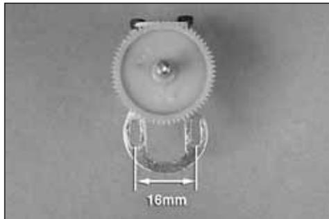
The ElectriFly Ammo motors have high kVs meaning that they like to run at very high rpm. A gear drive is used in order to reduce the rpm allowing a larger, more efficient propeller to be used. Great Planes ElectriFly offers a **20mm Stick Mount Gear Drive (GPMG0500)** with several pinions that allow for the following gear ratios:
