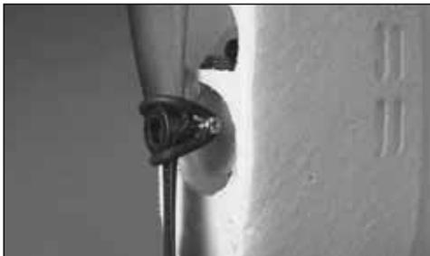
Install the prop on the prop hub and secure it with a rubber O-ring looped over both of the machine screws.
