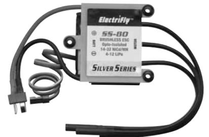
An ESC is basically the device that controls your motor through your radio system. Never run any RimFire motors with a brushed ESC. It will not work and you may damage both the motor and the ESC. Always use a brushless ESC. ElectriFly offers the **Silver Series SS-80 Brushless ESC (GPM1860)** or the **Silver Series SS-100 Brushless ESC (GPM1870)** that work well with the RimFire 1.60 (63-62-250) motor.
