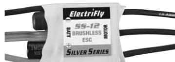
ElectriFly Silver Series 12 (SS-12) ESC (GPM1810) for 12A maximum constant current draw.
