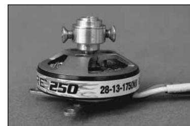
Install the cowl if the plane comes with one. Install the prop on the prop saver and secure it with a rubber O-ring looped over both of the machine screws. Check the O-ring for wear before each flight. If the O-ring shows any cracks, replace immediately.
