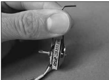
The motor can now be mounted from the back side of a firewall with only the shaft protruding forward of the firewall. The prop saver adapter or an optional collet or set screw type adapter can be used to attach the propeller to the motor.
