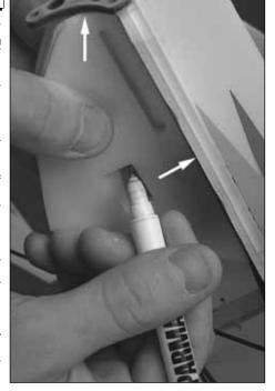
doubler that is required for the Firewall-Mounted installation. trace the template on one side of the plane. Trace the template with a fine marker or pen accordingly. Only  $\square$  2. Place the template directly over the bottom fuselage
