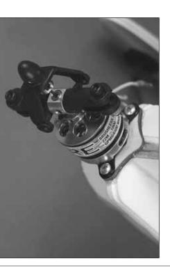
☐ 5. Install the V-Pitch and Rimfire motor onto the plywood firewall using (3) #4 x 3/8" wood screws (not included). Make sure the wire exits the slot correctly before tightening the screws. Apply a drop of foam safe CA to the screws to ensure they will not back out.
