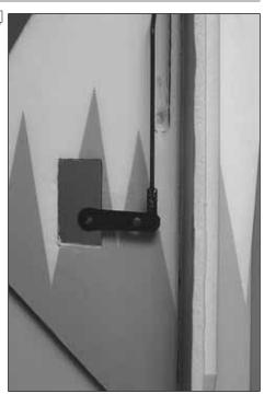
L 6. Locate one servo arm and a z-bend from your FlatOut parts tree. Clip the z-bend through the servo arm. Next, press the shaft into the z-bend as shown. After you have firmly pressed the shaft into the z-bend, apply a drop of foam safe CA to keep the shaft from slipping out.
