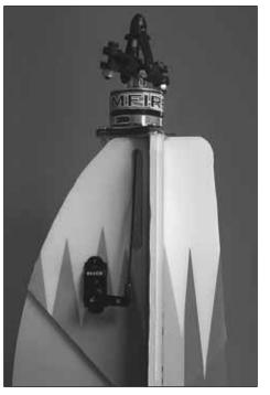
$\Box$  7. Install your servo into the slot as shown with a few drops of foam safe CA.
