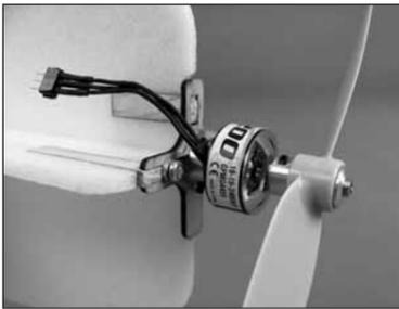
6. If you choose to use the "prop saver" attachment method, install the two M2 x 6mm countersunk machine screws in the prop adapter hub. Fit the prop and bushing (if needed) and fit the prop. Hook the rubber O-ring to one of the countersunk screws. Stretch it across the hub of the prop and hook it onto the other countersunk screw to retain the propeller. Use thread locking compound on all screw threads.
