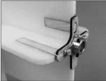
3. Fit the motor to the mount. Rotate the motor so that the motor wires can be routed in the desired direction. Install the two set screws using thread locking compound on the screw threads. With the motor in position, tighten the set screws securely.
