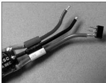
4. Mount the ESC to your model using double-sided tape or hook and loop material. Make sure that you choose a place that will allow all of the wires to reach. Plug the ESC signal lead into your receiver.
