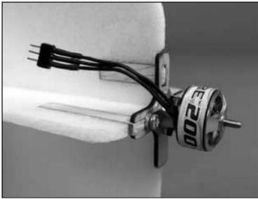
4. The prop adapter is stepped to fit 3mm and 4mm prop hubs. We have also included a 5mm and a 6mm bushing.
