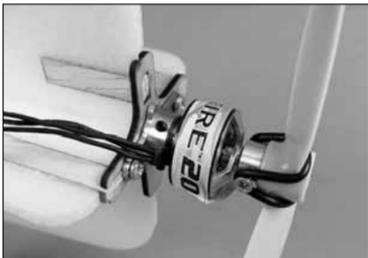
If mounting space is a concern, you can flip the motor mount around and decrease the amount of space you need to mount the motor. If you want to do this, use the template in this manual to help you grind away a hole to allow the motor mount to drop in.
