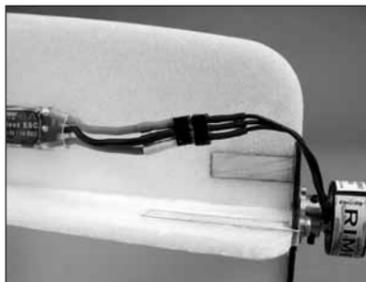
motor. If it does not rotate correctly, unplug the micro 3-pole connector and rotate it 180°. This will reverse the motor rotation.
