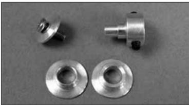
5. You have two options when installing the propeller. To install the propeller using the standard method, install the two set screws in the prop adapter hub. Fit the prop and bushing (if needed) and install the prop washer and screw. Use thread locking compound on all screw threads.
