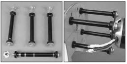
5. Select the mount base/spacer/bolt combination necessary to extend your motor the correct distance from the firewall. Apply a few drops of threadlocker to the threads on the end of the mounting bolts. Then, mount your motor using  $1/4^{"}$  [6.4mm] lock washers and  $1/4^{"}$  [6.4mm] flat washers under the heads of the bolts.
