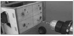
3. Drill 1/8" [3.2mm] guide holes through the firewall at the marks you made with the template. Then, enlarge the guide holes with a 9/32" [7.1mm] drill to accommodate the blind nuts.
