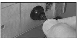
4. Use a 3/16" hex wrench to draw the blind nuts into the back of the firewall with one of the mount bases and a short 1/4-20 bolt. **Optional:** Apply medium CA around each blind nut to permanently hold it into the back of the firewall – use care **NOT** to get any CA into the threads.
