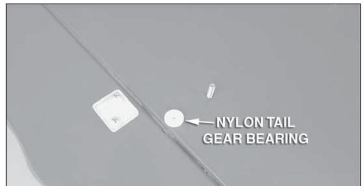
❑ 2. Apply CA or epoxy to the outside of the nylon tail gear bearing and insert it into the hole at the rear of the fuselage by gently tapping it into place until fully seated. Be sure not to get glue into the hole in the bushing.
