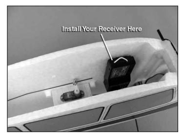
□ 2. Connect the elevator servo to the elevator channel on your receiver. Connect the rudder servo to the aileron channel on the receiver. Connect the ESC signal lead to the throttle channel on the receiver. Test for proper operation of all servos and the motor. If the motor rotates the wrong direction, unplug and swap the position of any two motor wires. Then, mount your receiver in the model using the piece of double-sided foam tape that was provided in this kit.
