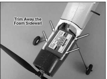
□ 4. The following two LiPo battery choices are now available. If you want to use the larger 640mAh battery, use a hobby knife to trim the side wall of the battery compartment to allow for easy installation and removal of the battery.
